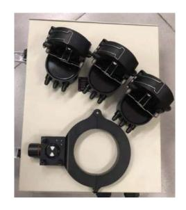
The DYX-FF Remote underground fault indicator is used in 6~35KV cable line distribution networks, it is usually installed in Ring Main Unit, Cable Distribution Box, Switch Cabinet, and so on, enable the maintenance engineers to identify the faulty section of network and restore power supply to customers on healthy sections in the shortest time.
