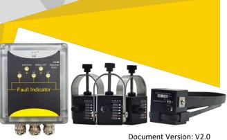
The earth-fault and short-circuit indicator type DYO-FF is used in 5~38KV cable line (underground) power distribution networks to monitor and locate earth fault and short-circuit. The red LED in display unit will blink when short circuit or earth fault happens. The fault information will also be sent to SCADA system by external connected IP Modem or RTU/FRTU.
