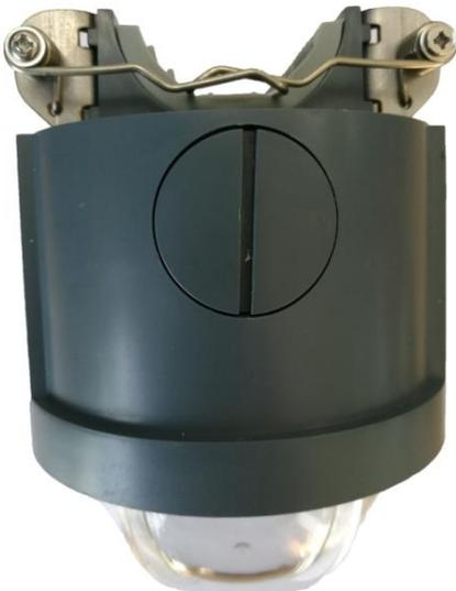
JJZ-HW-FI V1.0 Overhead Line Fault Indicators is usually used in 5~38KV overhead line power distribution network to monitor and detect short-circuit and earth fault. The fault signal is indicated by mechanical flag and three ultra-bright blinking LEDs with 360° sight.
