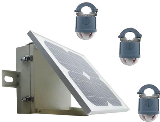
JYZ-FF-FI Overhead Line Remote Fault Indicators is usually used in 5~38KV overhead line power distribution network to monitor and detect short-circuit and earth fault. The fault signal is indicated by mechanical flag and three ultra-bright blinking LEDs with 360° sight. The fault information and load current value can also be uploaded to the SCADA by 2G/3G/4G networks.
