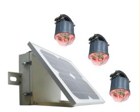
JYZ-HW-FI Overhead Line Remote Fault Indicators is usually used in 5~38KV overhead line power distribution network to monitor and detect short-circuit and earth fault. The fault signal is indicated by mechanical flag and three ultra-bright blinking LEDs with 360° sight. The fault information and load current value can also be uploaded to the SCADA by 2G/3G/4G networks.
