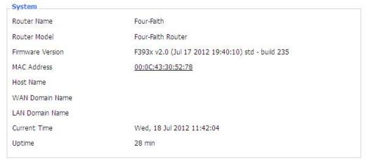
Router Name: name of the router, setting > basic setting to modify
