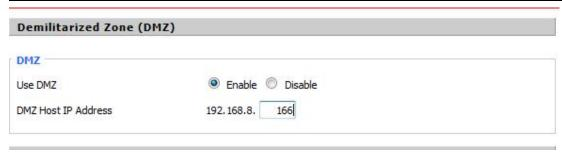
Any PC whose port is being forwarded must should have a new static IP address assigned to it because its IP address may change when using the DHCP function.
