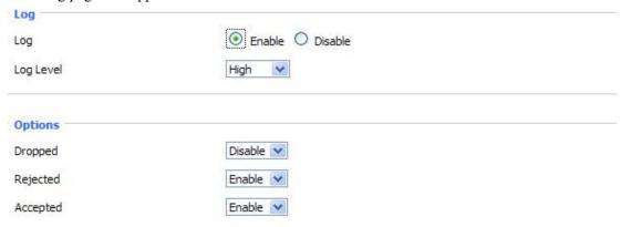
Log Level: Set this to the required log level. Set Log Level higher to log more actions.
