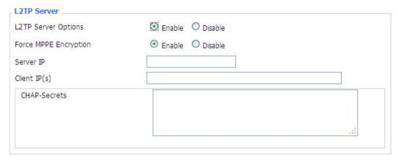
Force MPPE Encryption: enable or disable force MPPE encryption of L2TP data
