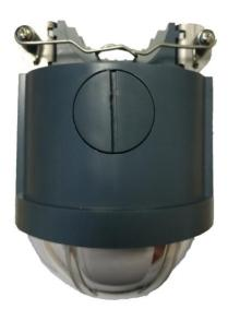
JJZ-FF-FI Overhead Line Fault Indicators is usually used in 5~38KV overhead line power distribution network to monitor and detect short-circuit and earth fault. The fault signal is indicated by mechanical flag and three ultra-bright blinking LEDs with 360° sight.
