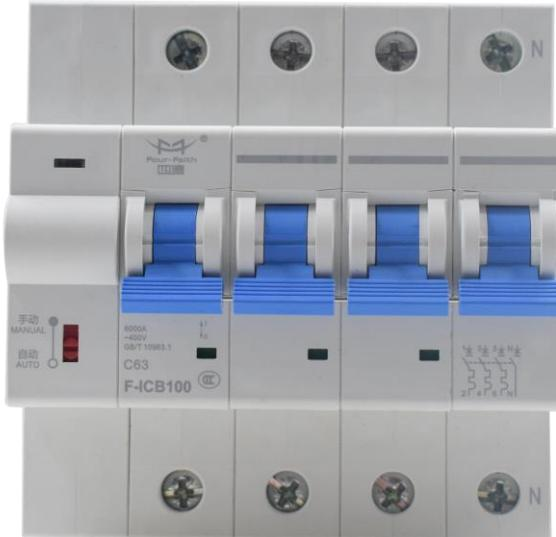
F-ICB100 is a smart MCB (Miniature Circuit Breaker), which integrates the functions of communication, control, current, voltage, leakage, temperature and power monitoring, realized real-time monitoring, warning, leakage detection and protection of 220V/380V power lines. It has high short circuit capacity. It can provide 1 / 2 / 3 / 4P products, which is widely used in general power supply system, unattended areas, substation and other scenarios.
