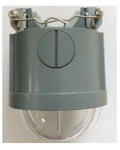
JJZ-FF Overhead Line Fault Indicator is usually used in 5~38KV overhead line power distribution network to monitor and detect short-circuit and earth fault. The fault is indicated by mechanical flag and three ultra-bright blinking LEDs with 360° sight.
