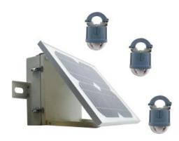
JYZ-FF Overhead Line Remote Fault Indicators is usually used in 5~38KV (can be customized by 44KV, 69KV and 110KV) overhead line power distribution network to monitor and detect short- circuit and earth fault. The fault signal is indicated by mechanical flag and three ultra-bright blinking LEDs with 360° sight. The fault information and current value can also be uploaded to the SCADA by 2.5G/3G/4G networks.
