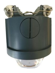
JJZ-HW-FI V1.0 Overhead Line Fault Indicators is usually used in 5~38KV overhead line power distribution network to monitor and detect short-circuit and earth fault. The fault signal is indicated by mechanical flag and three ultra-bright blinking LEDs with 360° sight.
