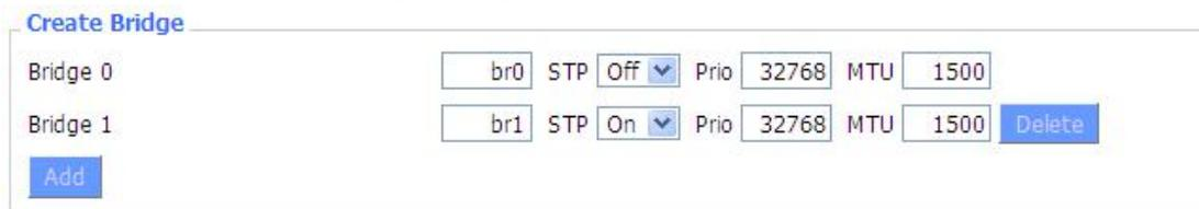
Create bridge option: the first br0 means bridge name. STP means to on/off spanning tree protocol. Prio means priority level of STP, the smaller the number, the higher the level. MTU means maximum transfer unit, default is 1500, delete if it is not need. And then click 'Save' or 'Add'. Bride properties is as below:
