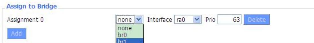
Assign to Bridge option: to assign different ports to created bridge. For example: assign port (wireless port) is ra0 in br1 bridge as below:
