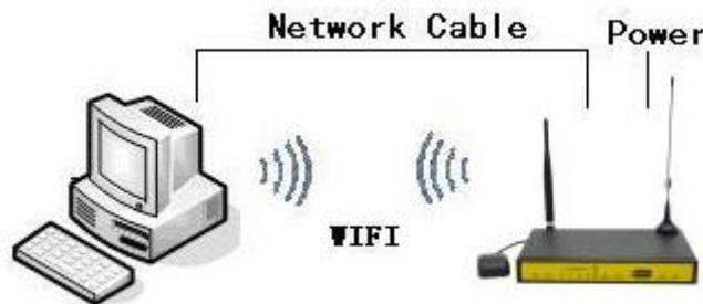
Please modify the IP address of PC as the same network segment address of the router, for instance, 192.168.1.9. Modify the mask code of PC as 255.255.255.0 and set the default gateway of PC as the router's IP address (192.168.1.1).
