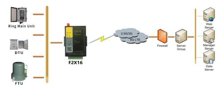
In the power distribution network system, where serial-based devices need data communication to the remote control center, using Four-Faith F2X16 Modem which also with Serial port and embedded with GPRS/3G/4G LTE module, enable the Electric Power Devices, such as Ring Main Unit, DTU and FTU to connect to the Remote Control Center over the cellular network, thus achieve remotely wireless data communication and monitoring.
