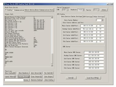
After Re-power IP MODEM, The configure tool will make it enter configure state. At the same time, the software will load current settings from IP MODEM and displays on the right configure columns. It's now ready to configure.
