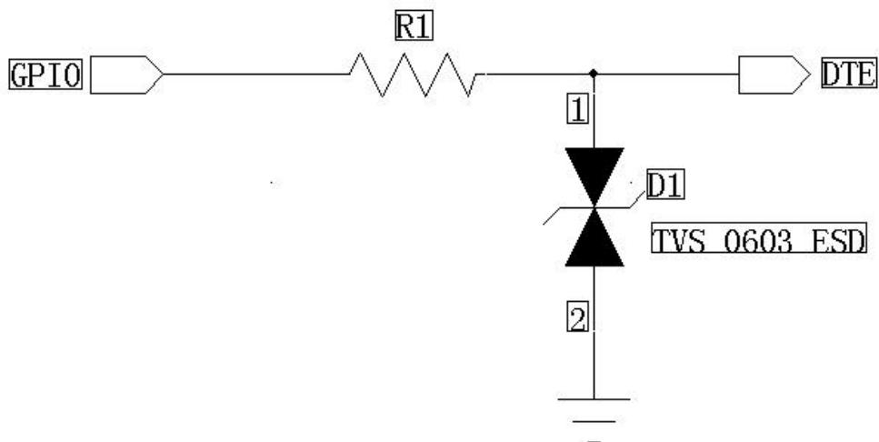
**Figure 5-5 TVS protection circuit for digital pin**
