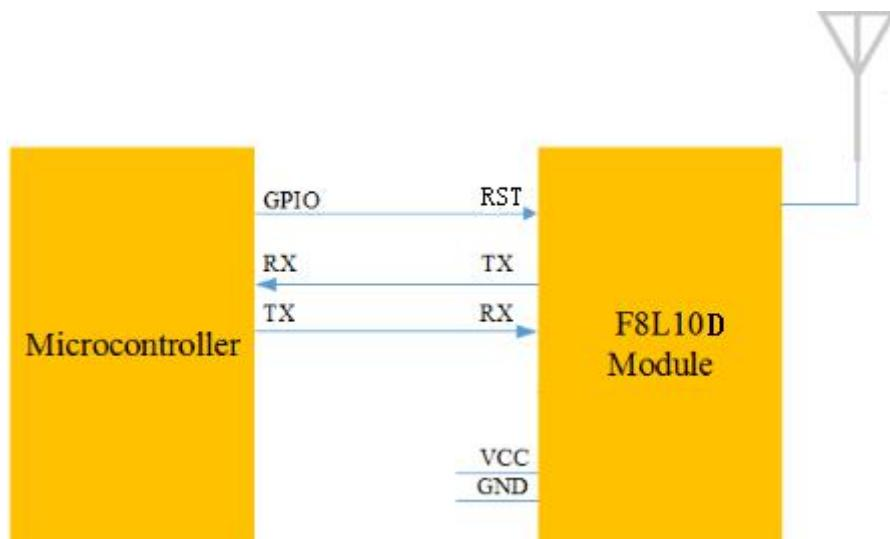
Figure 3-1 UART connection diagram
