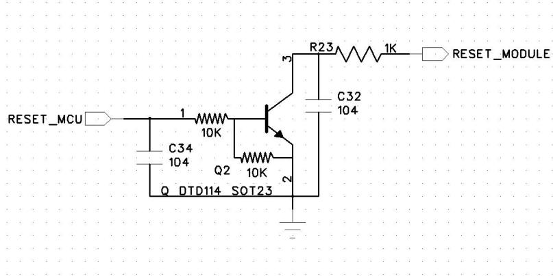
**Figure 5-4 MCU Control Triode Reset Reference Circuit**
