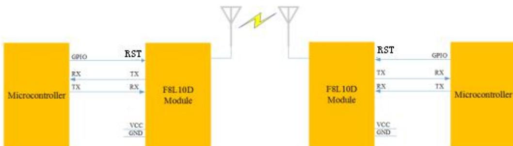
Figure 3-2 The UART convert to RF system
