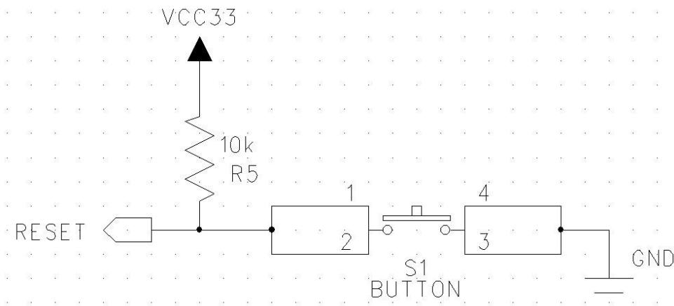
**Figure 5-3 Reset Circuit**
