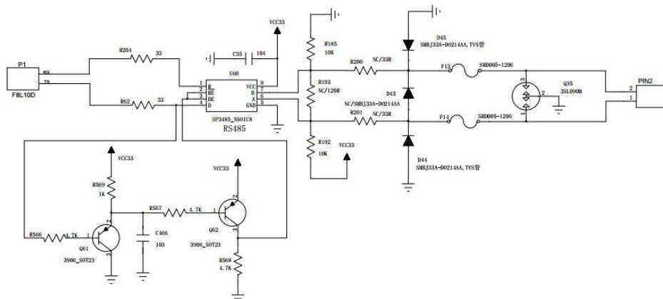
**Figure 5-2 F8L10D and IPC RS485 connection reference circuit**
