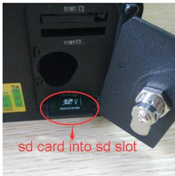
SD card must Make sure insert to the end of slot.
