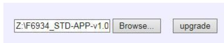
Check the “Browser” button, select the upgrade file ,check “upgrade” button to upgrade the device firmware.
