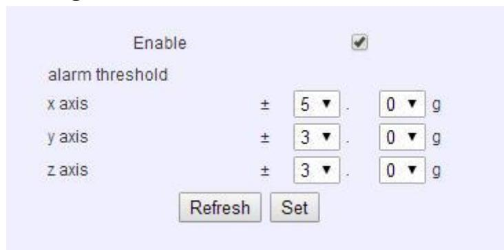
This dialog box configures g-sensor alarm thresholds. It has an 'Enable' checkbox (checked) and three sets of threshold sliders for X, Y, and Z axes. Each set consists of a ± range slider and two numerical input fields for the lower and upper limits in g-force units. It includes Refresh and Set buttons.
