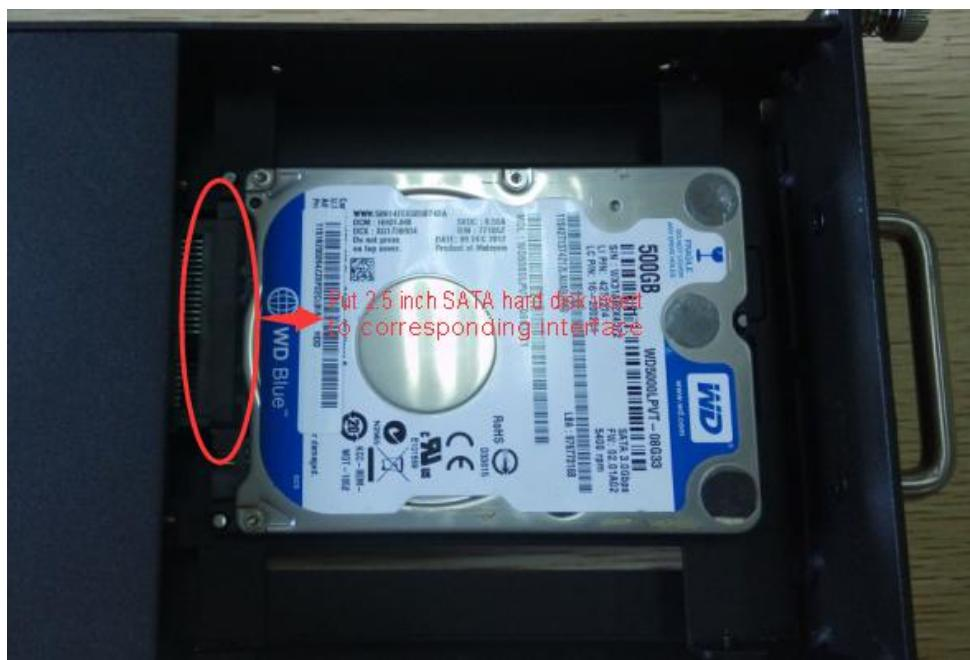
Lock the hard disk with 4 M3\*5 screw 。
