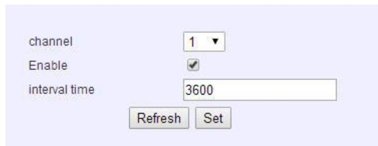
This dialog box allows configuration of a capture task. It includes fields for channel (set to 1), enable status (checked), and interval time (set to 3600 seconds). It also features Refresh and Set buttons.
