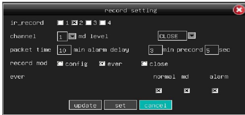
Ir\_record: check ir control key “rec” start or stop ir record .
