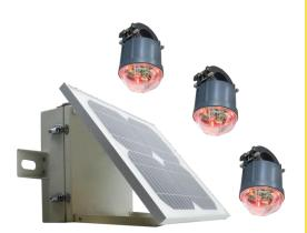
JYZ-HW Overhead Line Remote Fault Indicators is usually used in 5~38KV (can be customized by 44KV, 69KV and 110KV) overhead line power distribution network to monitor and detect short- circuit and earth fault. The fault signal is indicated by three ultra-bright blinking LEDs with 360° sight. The fault information and current value can also be uploaded to the SCADA by 2.5G/3G/4G networks.
