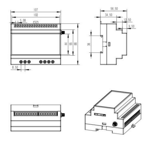
A.2 Terminals (18PIN spacing 5.08mm,3PIN spacing 8.5mm, 4PIN spacing 8.5mm)
