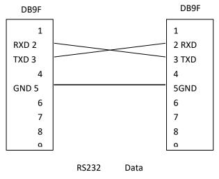
The signal connection of the RS232 data cable is as follows:
