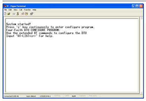
7. IP MODEM has entered configure state, you can configure the parameters through AT command.
