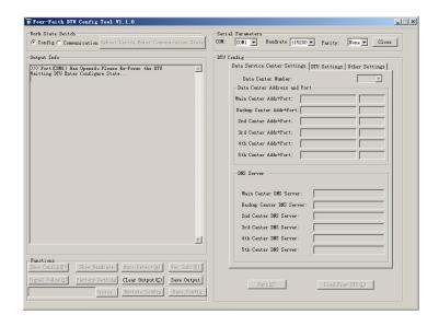
The "Serial Parameters" column shows the current serial port settings. To configure IP MODEM, please choose the correct serial port which connects to IP MODEM, and the baudrate is 115200 with no parity, then open the serial port. If the button text is "Close", it shows the serial port now has been opened. If the text is "Open", you should open the port first. When the port opened, the "Output Info" column will display
